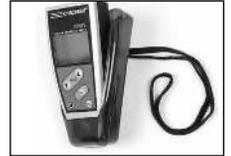
3. Place your thumbs on top corners of the gauge. Use your forefingers to slip the top corners of the shell over the top corners of the gauge.
