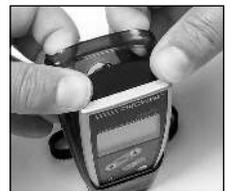
4. Check the bottom of the gauge to be sure that the measurement sensor is unobstructed and adjust the shell if needed.
